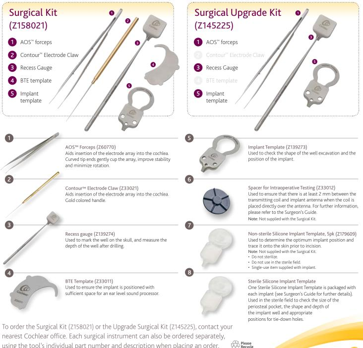
using the tool's individual part number and description when placing an order.
