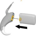
1 Align the battery module to the processor socket to fit the parts together.
