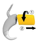
1 Twist the battery module as shown to remove it from the processing unit.
