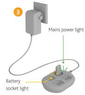
Angle and fit the rechargeable battery module into a socket on the Cochlear™ Nucleus® Battery Charger.
