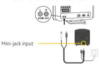
Connecting the TV Streamer to an analogue audio source using a headphone mini-jack adaptor.
