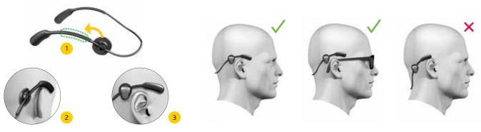
The Baha SoundArc should be placed just above the ears and follow the contours of the head.
