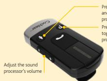
Press once to mute and unmute the sound processor's microphones. Press one or more times to toggle through the sound processor's programs
