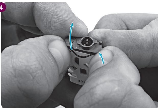
Then, pushing with your other thumb nail, create a loop in the O-ring, and ease the O-ring off.
