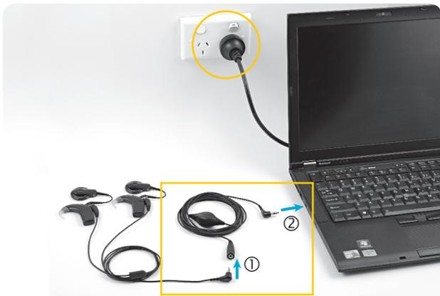
Connect a bilateral personal audio cable to the mains isolation cable in the same way.
