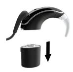
2. **Press and hold** the button (1) while reconnecting the battery (2).
