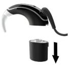
2. Pull the battery module from the processing unit.
