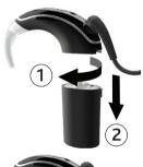
Twist to disconnect, then remove the battery module.
