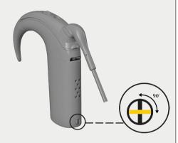
LOCK Turn the locking screw **clockwise** with the
