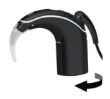
Twist the battery module as shown to release it from the processing unit.
