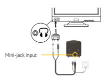
Connecting the TV Streamer to an analogue audio source using a scart adapter.
