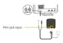
Connecting the TV Streamer to an analogue audio source using a headphone mini-jack adaptor.
