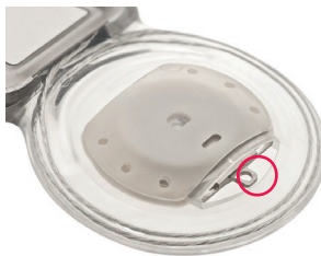
Figure 26: CI600 Series implant - metal tab on magnet cassette
