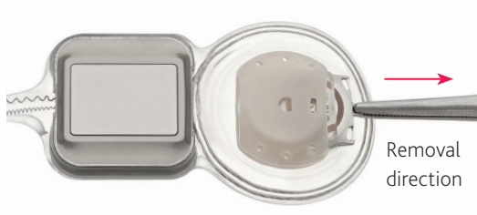
Figure 27: CI600 Series implant - magnet cassette removal using metal tab
