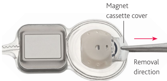
Figure 30: CI600 Series implant with magnet cassette partially removed
