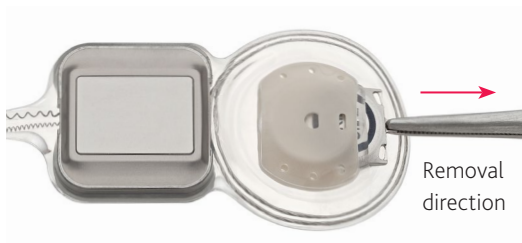
Figure 32: CI600 Series implant - magnet cassette removal using metal tab
