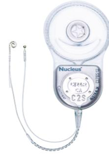
The CI24R was released in 2000 with perimodiolar (Contour Advance®) and straight electrodes.
