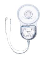
The CI24R was released in 2000 with perimodiolar (Contour Advance®) and straight electrodes.
